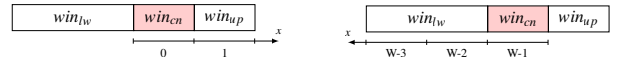
(a) Window is at the left border ( x=0 ). Border handling is necessary for the datum in win_{lower} .
